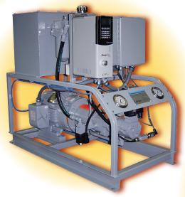
**Custom Power Units** are fabricated to meet exact customer requirements, with flows to 200 gpm (757 L/min) and pressures to 15 000 psi (1040 bar). Select prime movers to 400 HP (298 kW) and reservoirs to 1000 gallons (3785 L).
