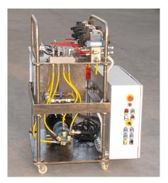
Test systems use Split-Flow® four-outlet PF1000 Series pumps for simultaneous testing of four components.
