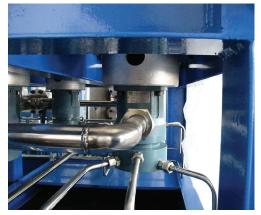
PF3000 Series pumps with four outlets operate at high pressure on lubrication systems. These Split-Flow® pumps simplify the circuit with less components and piping.
