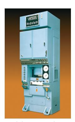
Dynex high pressure pumps have been used on industrial presses since 1960. Some pumps, operating at pressures to 15 000 psi (1040 bar), have been in use for 60 000 hours without failure.
