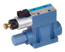
**HP05H** Directional Control Valves provide high pressure, high flow capability. The valve's low pressure drop is enhanced with the use of the Dynex standard subplate, which takes advantage of the valve's special double tank port design.
