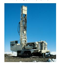
Variable delivery PV6000 Series pumps used on drill rigs power the drill rotation, drill pressure, mast movement, and propulsion. They've proven to be rugged and reliable even when subjected to shock, vibration, and long duty cycles.
