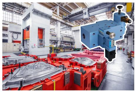
A custom designed, multi-function control system which replaces multiple components on a hydroform press retrofit application.
